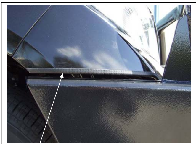
Figure 12: 3mm clip lock trim on outer cut edge of plastic bumper.
