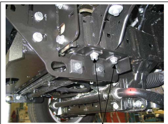
Figure 6: Note placement of 40 x 40 steel washers. Winch bracket shown in place.
