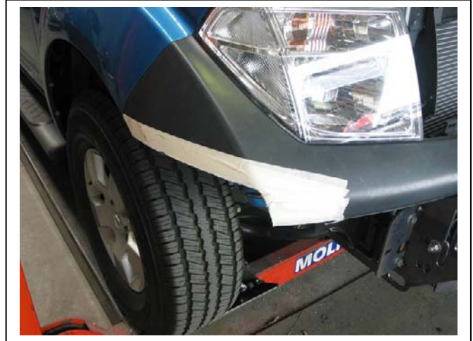
Figure 3: Use a sharp knife to cut front of bumper along crease line.
